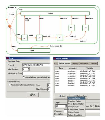
Figure 1: Safety task consisting of system model, safety requirement and injected failures.
